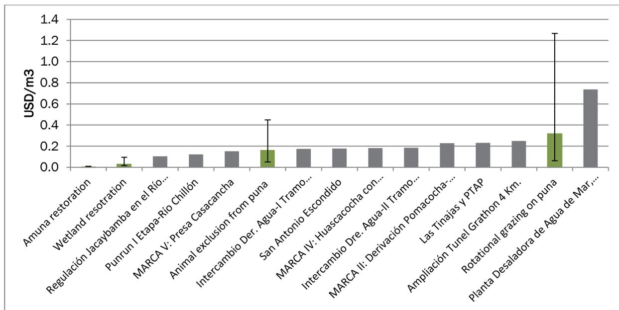
Figure 4. Costs (USD/m<sup>3</sup>) of green and gray interventions for Lima's water supply. Sources: current analysis and Nippon Koei (2011).
