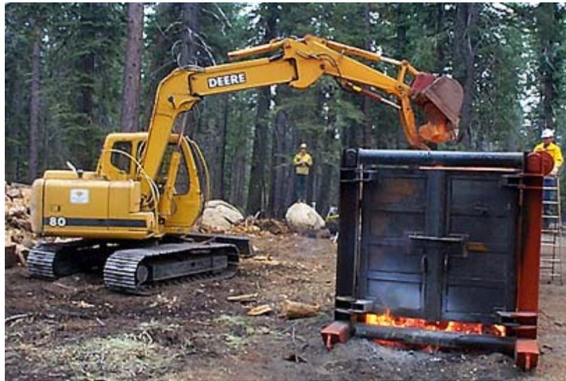
**Figure 16. Air curtain burner.**
