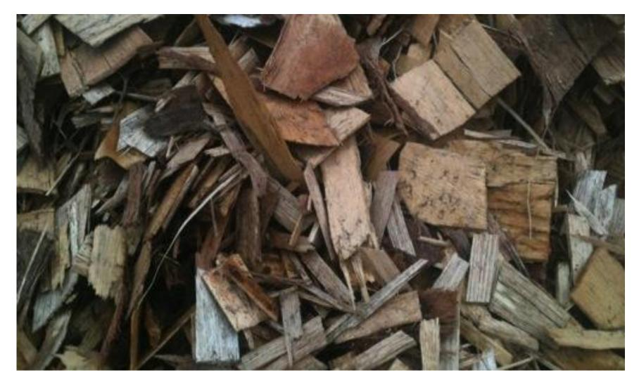
Waste materials from primary and secondary processing are often used as input materials for the production MDF and particle board
