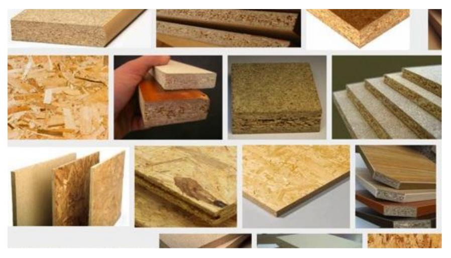
Particle board is a cheaper, denser and more uniform than conventional wood and plywood and is substituted for them when appearance and strength are less important than cost.
