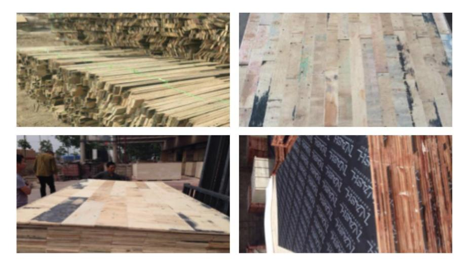
Reclaimed materials are process and combined with (non-recycled) face and back veneers for the production of plywood
