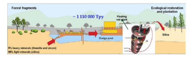
Figure 30: Process of ilmenite mining in Madagascar
