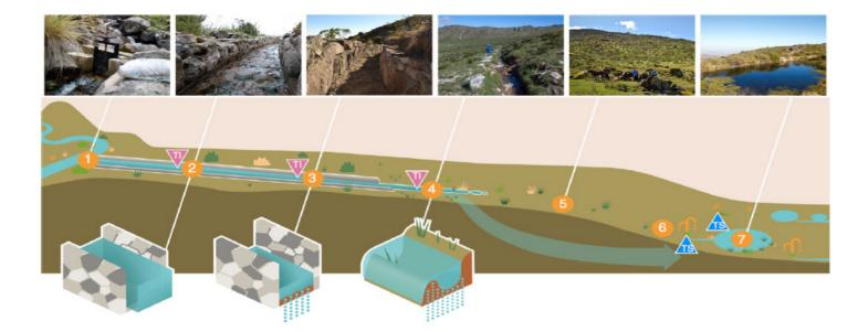
**Conceptual model of the pre-Inca infiltration enhancement system.** Features of the system: diversion canals (1 and 2), infiltration canals (3 and 4), infiltration hillslopes (5), springs (6) and ponds (7). Tracer injection (TI) and sampling (TS) points are marked schematically in the diagram.
